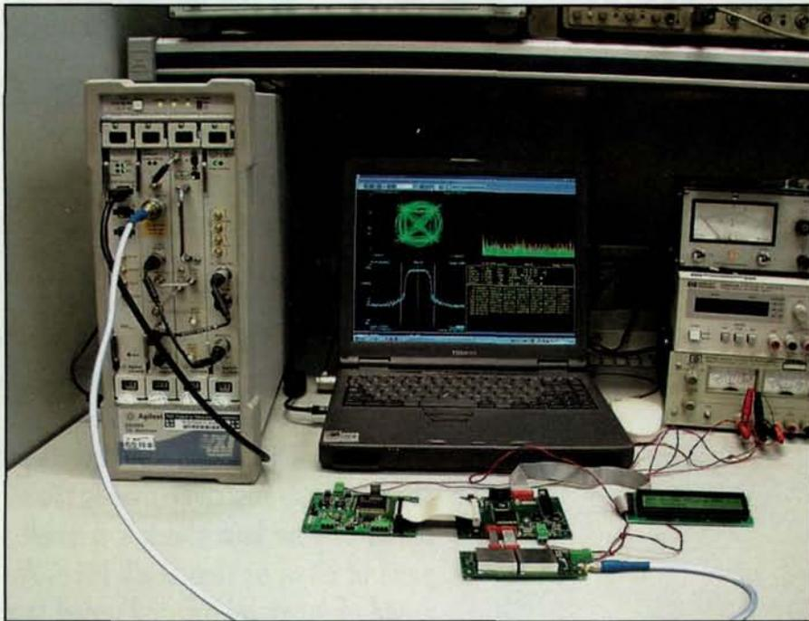
Photo A—The Dutch D-ATV boards under test. In front of the laptop computer are (from left to right) the MPEG-2 encoder, the DVB-S baseband encoder, and (toward the front) the transmitter. Note the LCD display, which is used by the DVB-S encoder to display status. (Photo courtesy of Henk, PE1JOK)
